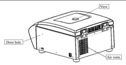
Figure 5.2 D1536 back view of the centrifuge
