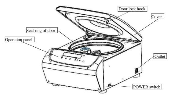
Figure 5.1 D1536 Front view of the centrifuge
