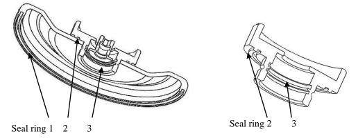
rings may fall off or aging after several autoclaving, need to be replaced or re-installed.
