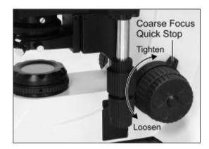
• To loosen the upper limit, just turn the lever in the opposite direction
