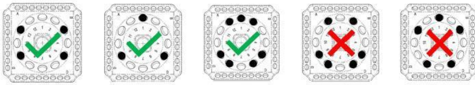
Figure 3. Examples of balanced (✓) and unbalanced (✗) loading.
